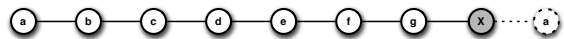
Fig. 10. Link Spoofing: The malicious router X advertises a spoofed link to router a in its TC messages, thus all routers will record the links X-a and b-a .
