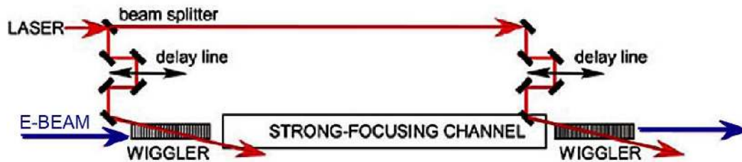
Figure 23. The laser conditioning scheme of Zholents is derived from the Vinokurov scheme. While experiments have been proposed to demonstrate the predicted benefits of beam conditioning, this exciting prospect awaits a definitive test.
