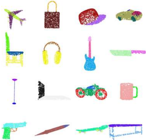
Figure 3. Part Segmentation Results on ShapeNet. Note that Car and Motor have lower performance than most other categories in Table 2. This is partly because there are more parts in these categories: 4 labels for Car and 5 labels for Motor .
