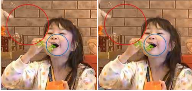
Fig. 13. Screenshot illustrating visual quality improvement from SAO for PartyScene @ 1.13Mbps with VTM-9.0 and ALF disabled in LDP case: (left) SAO off, (right) SAO on.
