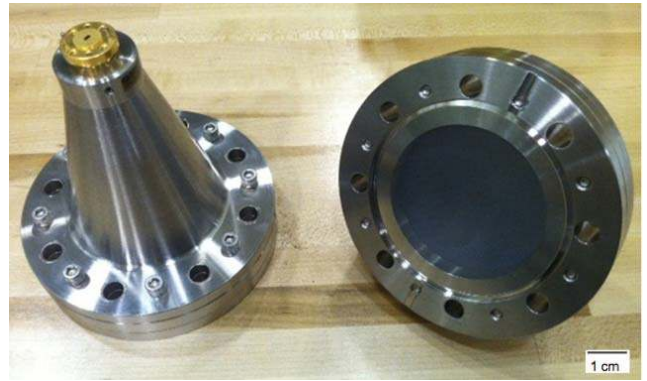
Fig. 3. Photograph of millimeter-wave, spot-focusing antennas, each with a WR-10 connector and interface compatible with either a vacuum chamber or open air.
