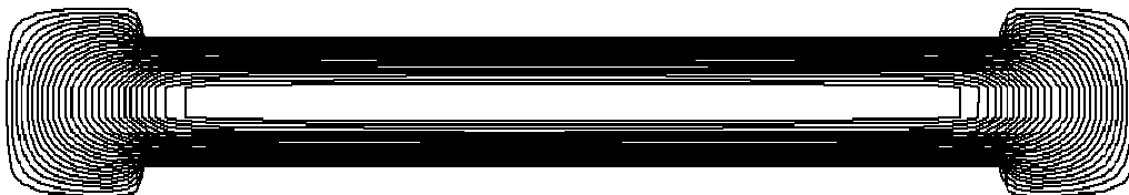
FIGURE 4. Contour plot of E_z(x,y) ; the beam motion is into the page.
