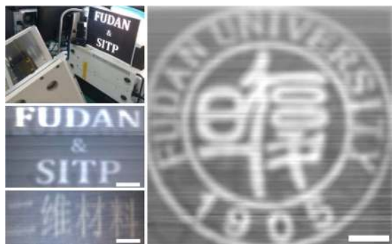
Figure 5 Experimental set-up and image acquisition by GaTe/Si photodiodes. The left upper panel shows the experimental set-up, including the piezoelectric platform, camera, and target. All the other panels are the images taken by the GaTe/Si diodes with reasonable contrast and spatial resolution: “Fudan & SITP”, “two-dimensional material” (in Chinese), and an official logo of Fudan University. The scale bar is 50 mm.
