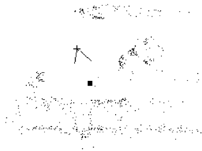
Figure 5: Bird's eye view of the SIFT map around base region: the home location is indicated by the square with the current robot position and view direction shown as a V.
