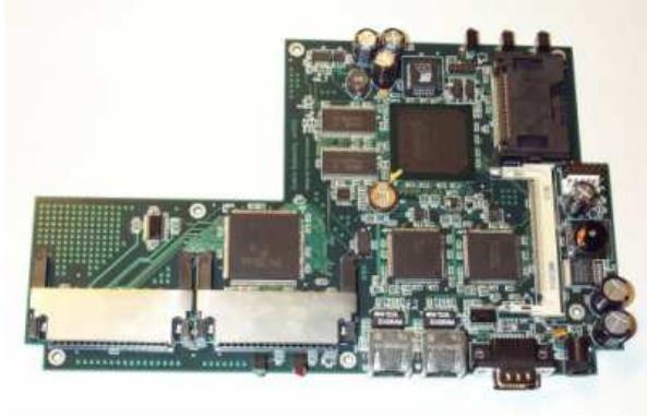
Figure 2: The Soekris net4521 single board computer
