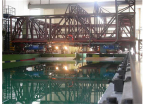
FIG. 1. A front view of the carriage of the University of Naples Federico II towing tank.
