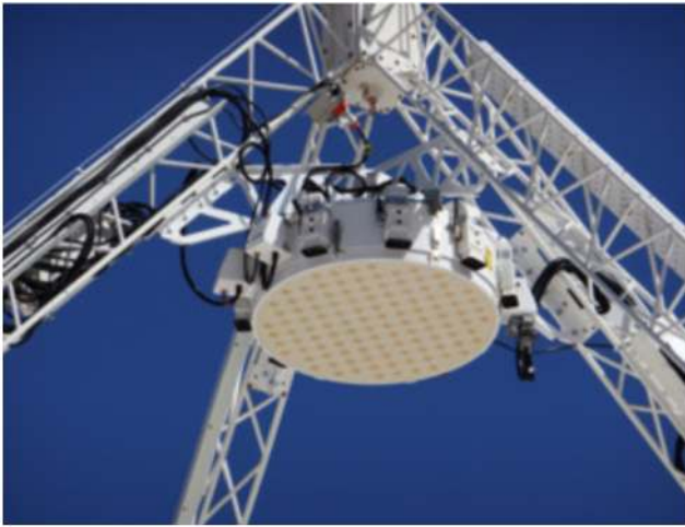
Fig. 2 Second-generation ASKAP Phased Array Feed (Chippendale et al. 2014), used to form 36 beams providing a \sim 30 sq deg field-of-view at 1.4 GHz, ideal for widefield 21-cm sky surveys. — Photo Credit: CSIRO
