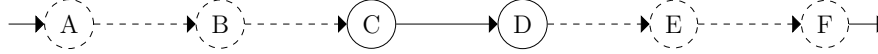
Fig. 6. Partial / incomplete traces: events “A”, “B”, “C”, “D”, “E”, and “F” have occurred in reality. Only events “C” and “D” are included in the log whereas the prefix with events “A” and “B” and the suffix with events “E” and “F” are not included.
