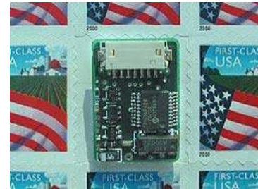
Figure 3.11 – SenseWear transceiver module
