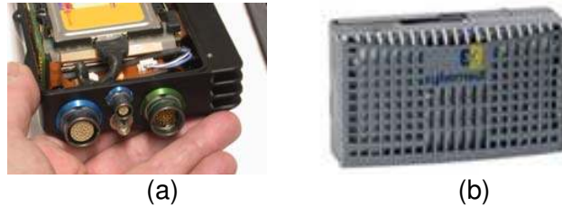
Figure 10.1 – (a) Infologix ViA II Super Rugged with Caruso Transmeta processor (b) Xybernaut Mobile Assistant V with Celeron ultra-low voltage processor
