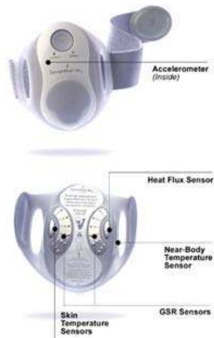
Figure 3.10 – SenseWear embedded sensors
