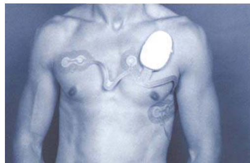
Figure 3.2 – Nexan sensor patch and wireless transceiver
