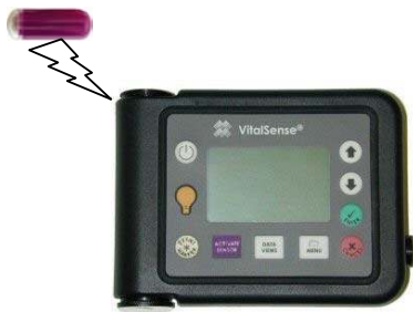
Figure 4.6 – Ingestible core body temperature capsule (Jonah™) and multichannel RF receiver and data logger (VitalSense) from Mini Mitter
