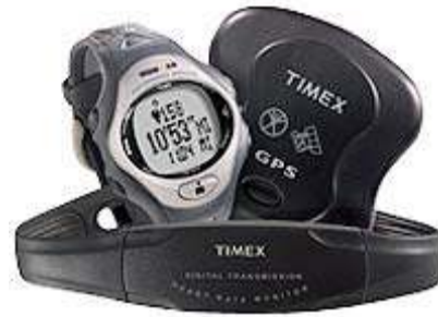
Figure 3.13 – Timex digital FM heart rate and GPS time and distance performance monitoring system
