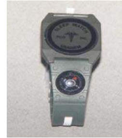
Figure 4.9 – Actigraph wristwatch with integral skin temperature sensor. (Precision Control Design, Ft. Walton Beach, FL)
