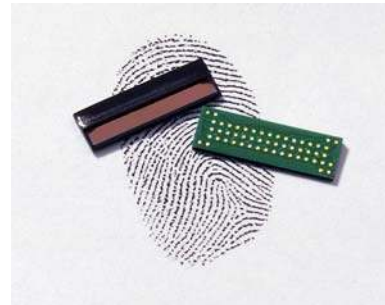
Figure 4.14 – Fujitsu MBF300 fingerprint sensor array
