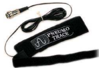
Figure 4.5 – ADInstruments respiratory belt transducer
