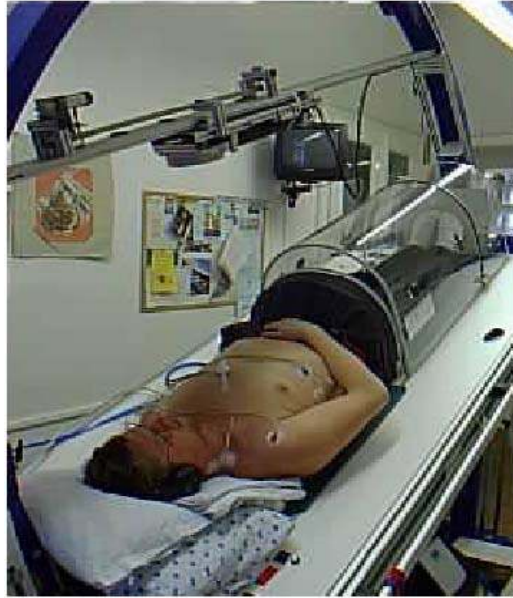
Figure E.5 – An LBNP chamber used to study the cerebral hemodynamic response to posturally simulated microgravity, as experienced during spaceflight
