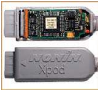
Figure 3.3 – Nonin Xpod oximetry module
