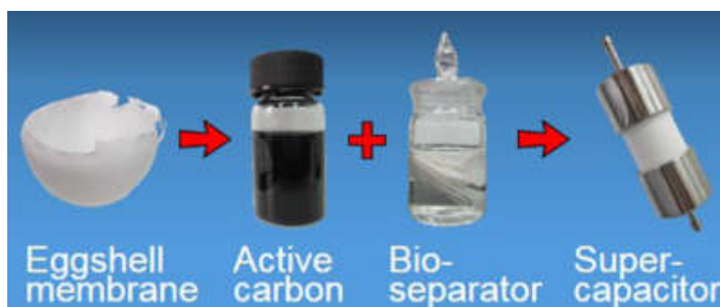
Figure 24. Fabrication of an asymmetric supercapacitor using biowastes-derived materials from chicken egg shells. Adapted with permission from ref. 184.
