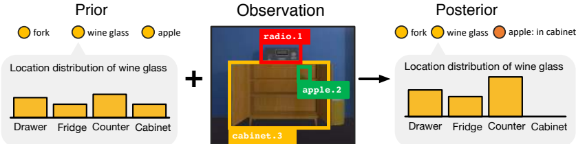
Figure 13: The agent’s belief is represented as the location distribution of objects, and is updated at each step based on the previous belief and the latest observation. In the example, the open cabinet reveals that the wine glass can not be in there, and that there is an apple inside, updating the belief accordingly.
