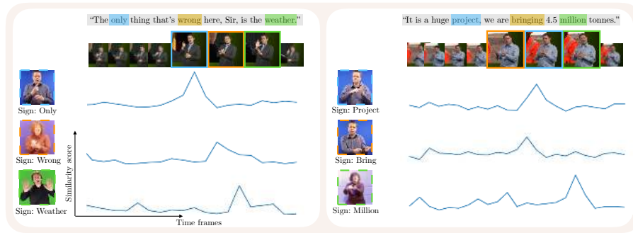
Fig. 6: Densification: We plot the similarity scores between BSL-1K test clips and BSLDICT examples over time, by querying only the words in the subtitle. The predicted locations of the signs correspond to the peak similarity scores.
