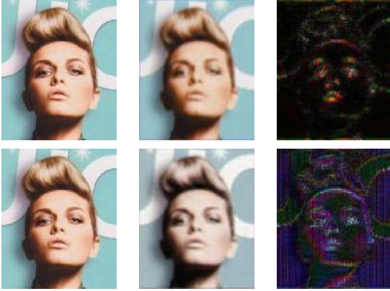
Figure 6: Effects of spectral distortions on the image outputs in our simple AE setting. Left: original image; Center: AE output image; Right: filtered difference image. The top row shows the blurring effect of missing high frequencies in the (up+conv) case; Bottom row shows the high frequency artifacts induces by (transconv).
