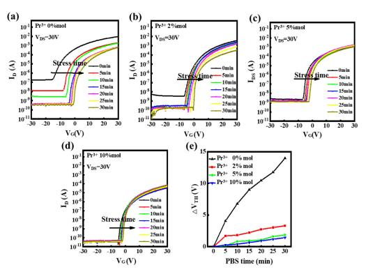
**Figure 9.** Transfer curves variations under positive bias stress for In-Pr-O TFTs with Pr mol% ratios of (**a**) 0 mol%, (**b**) 2 mol%, (**c**) 5 mol%, (**d**) 10 mol%, and (**e**) summary of  $V_{\rm T}$  shifts.
