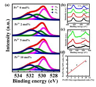
**Figure 7.** X-ray photoelectron spectroscopy spectra for In-Pr-O films with indicated Pr concentrations. (a) O 1s, (b) In 3d, (c) Pr 3d, and (d) Pr doping ratio between solution and thin film.
