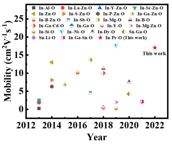
Figure 11. Recent advances of sol-gel oxide TFTs on Si/SiO<sub>2</sub> substrate.
