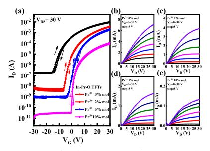
**Figure 8.** (a) Transfer and (**b**–**e**) output curves for In-Pr-O TFTs with 0, 2, 5, and 10 mol% Pr concentrations.
