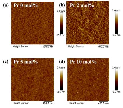
**Figure 4.** Images of In-Pr-O films with With Pr ratios of (**a**) 0, (**b**) 2, (**c**) 5, and (**d**) 10 mol% by atomic force microscopy.
