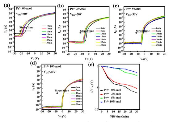
**Figure 10.** Transfer curves variations under negative bias stress for In-Pr-O TFTs with Pr mol% ratios of (**a**) 0 %, (**b**) 2 %, (**c**) 5 %, (**d**) 10 %, and (**e**) summary of  $V_{\rm T}$  shifts.
