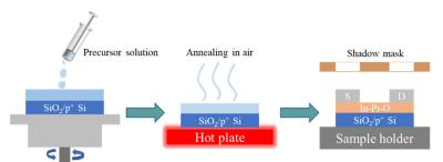
Figure 1. Schematic showing the fabricated In-Pr-O TFTs.
