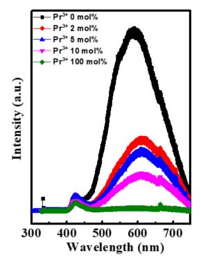
Figure 6. Photoluminescence spectra for In-Pr-O with indicated Pr concentrations.
