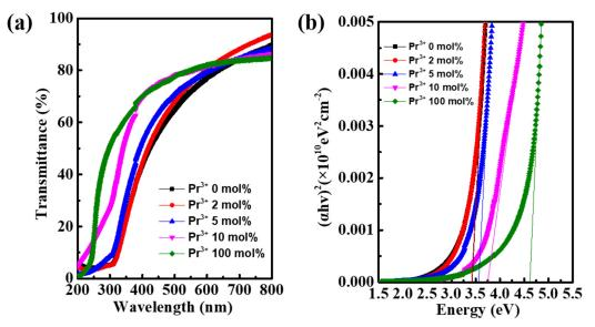
**Figure 5.** (a) Transmittance spectra and (b) evaluation of optical bandgap for In-Pr-O layer with different Pr ratios.
