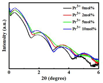
Figure 3. X-ray reflectivity patterns of In-Pr-O films with various Pr contents.
