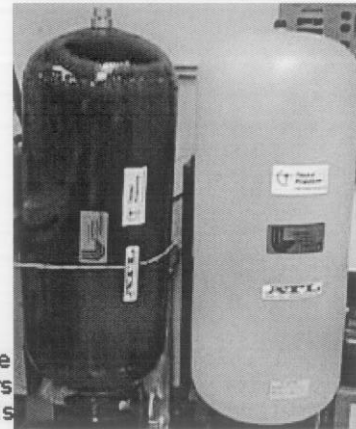
Figure 4. Lightweight Bladder-Lined Tankage was Prototyped using Molded or Fabricated Liners
