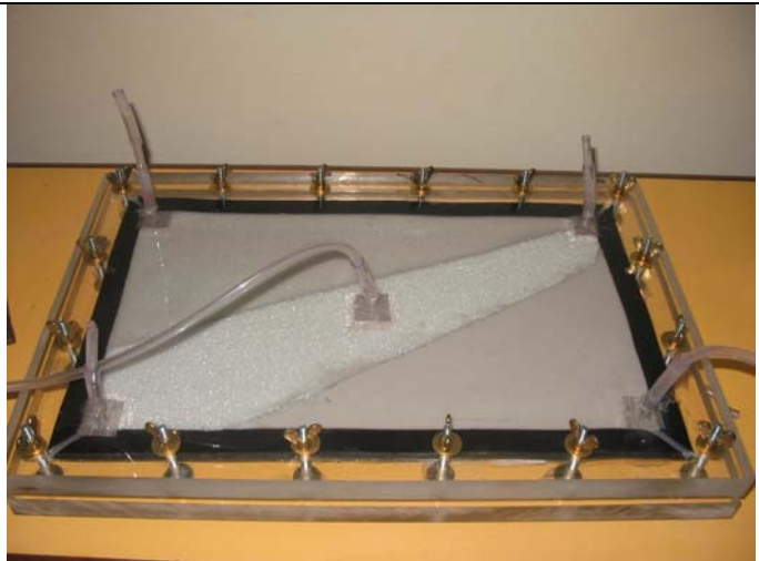
Fig. 4: Final situation. Zone 1 at S_{wirr} while Zone 2 is still at S_w=100\% . No transition zone is generated. FWL has no physical meaning
