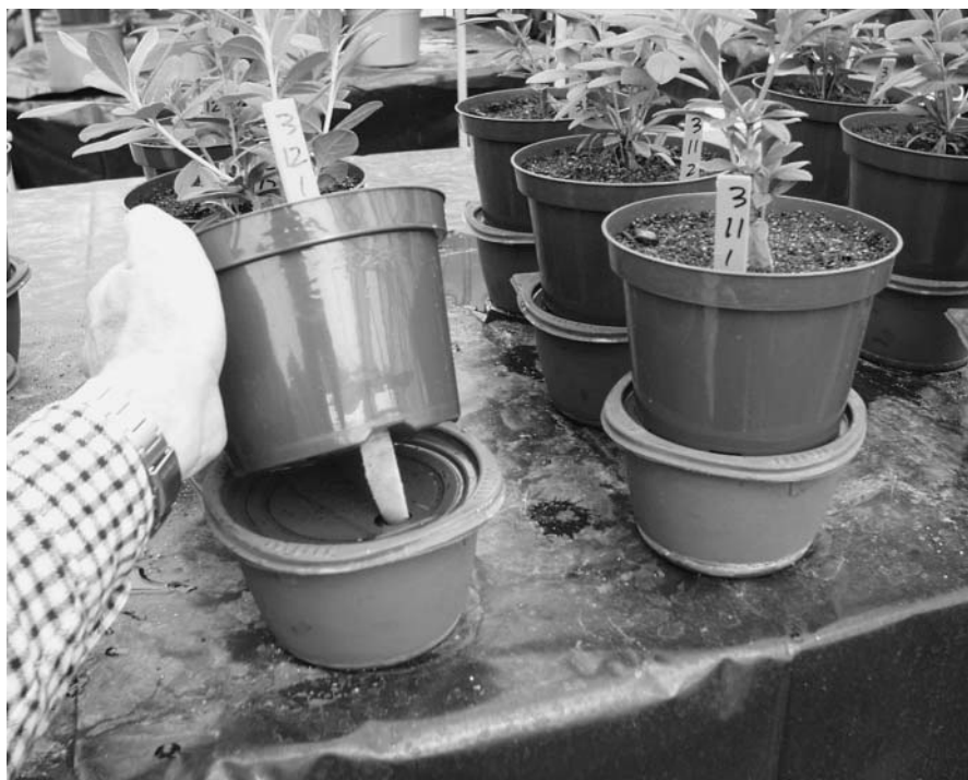
Fig. 1. The wick irrigation assembly consisted of a 6.5-inch-diameter (16.51 cm) “azalea” container placed over a water-filled, 1-L (0.26-gal) plastic reservoir with a 0.75-inch-diameter (1.91-cm) hole cut in the lid. An absorbent wick positioned along the inner wall and out a drain hole of the container extended into the reservoir through the hole in the lid to allow for continuous capillary wetting of the container substrate.
