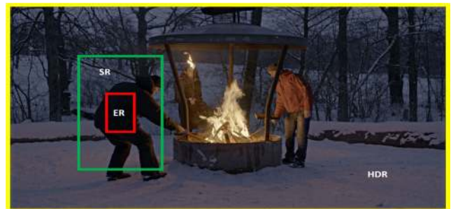
FIGURE 11. Regions used to compute the luma variation thresholds. ER is the m \times n embedding region. SR comprises the eight m \times n blocks surrounding ER. HDR comprises all pixels locations except for those in ER and SR.
