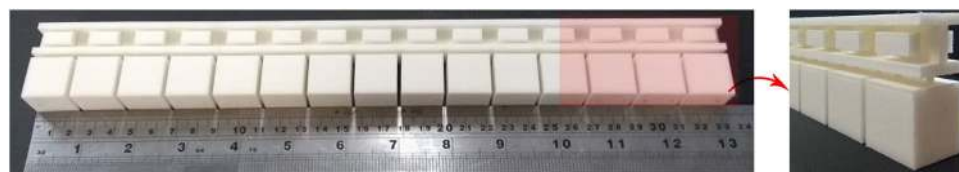
Figure 3. Metamaterial beam with attached cube specimens constructed in SLS 3D printing.
