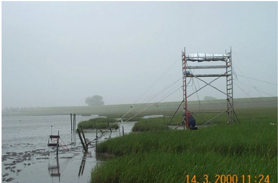
Figure 3.4: A ‘logger tower’ and some gauges near the edge of the salt marsh.
