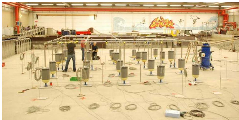
Figure 5. Construction of WEC support structures in the DHI wave basin.
