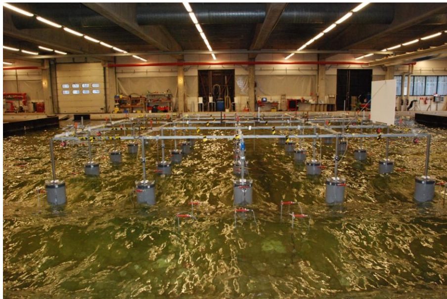
Figure 14. The 5 \times 5 -WEC rectilinear array in the DHI Shallow Water wave basin, under irregular long-crested waves with \theta = 0^\circ . View from behind the wave generator.
