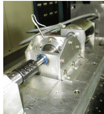
Figure 2b: Assembled thrust and torque transducers.
