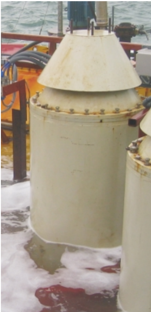
Figure 6: Kaplan turbine with cylinder gate.
