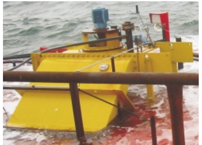
Figure 5: Kaplan turbine with Siphon inlet
