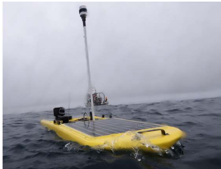
Fig 2. Wave Glider SV2. (Top) Blow-out showing the near-surface float housing the payload (including an ADCP (blue) and fluorometer), and connected to a sub ('glider part'). The wave-induced friction between the two parts, connected through an umbilical, provides thrust. (Below) The Wave Glider in operation showing the antenna and solar panels. (Pictures courtesy of Liquid Robotics Inc.).
