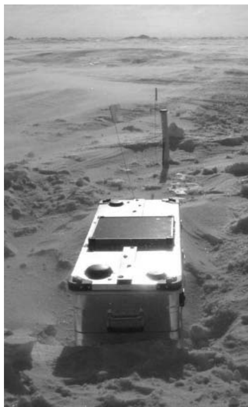
Fig. 3. A tiltmeter buoy deployed onto the multi-year floe at the ice camp. The large square solar panel is clearly visible, as is the second GPS antenna mounted atop a separate pole, furthest from the camera. The Iridium (left) and GPS (right) antennae can be seen on the top of the box nearest the camera. The box is sitting on the hard ice surface beneath the snow.
