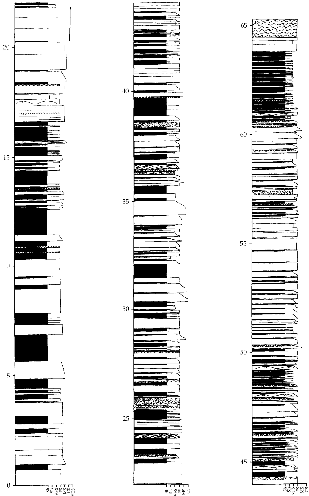
FIG. 9.—Stratigraphic section from Heale Peak dominated by thin- to medium-bedded sandstone and shale facies.
