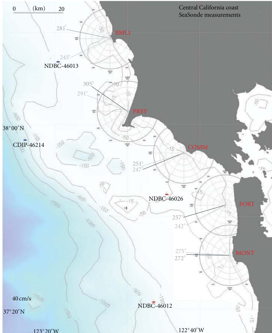
FIGURE 16: Annual mean wave directions for 2007 calculated from SeaSonde wave data (dark grey) and near-shore CDIP model annual mean wave direction results (light grey).
