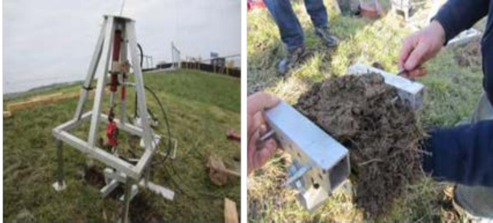
Figure 16. The sod pulling device (left) and the pull frame with a sod pulled from the grass cover.
