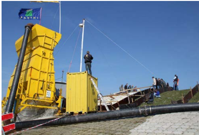
Figure 2. The Wave Overtopping Simulator used in a pilot test on wave run-up simulation.
