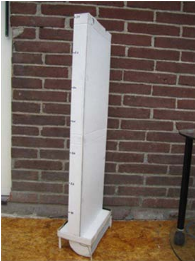
Figure 4. Small scale model of first design of the Wave Run-up Simulator.
