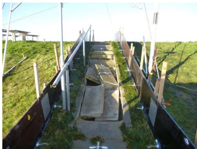
Figure 9. Testing a staircase with wave run-up simulation.
