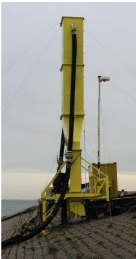
Figure 6. Wave Run-up Simulator seen from the side.
