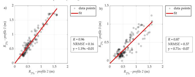
**Figure 11.** (a) Relationship between the wave runup,  $R_{2\%}$ , measured on the centerline profile (profile 2 in Figure 1d) and westward profile (profile 1 in Figure 1d); (b) Relationship between the wave runup,  $R_{2\%}$ , measured on the centerline profile (profile 2 in Figure 1d) and eastward profile (profile 3 in Figure 1d).
