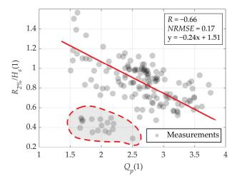
**Figure 9.** Scatter plot of relative run up  $(R_{2\%}/H_s)$  against Goda peakedness parameter  $(Q_p)$  on the centerline profile (profile 2 in Figure 1d) on the fetch-limited gravel beach; the area enclosed by a red dashed line marks a cluster of data points that exhibit specific swash behavior, which occurs at highly oblique wave directions, low tides, low significant wave heights, and low wave spread. Detailed information can be found in the text in Section 3.3.
