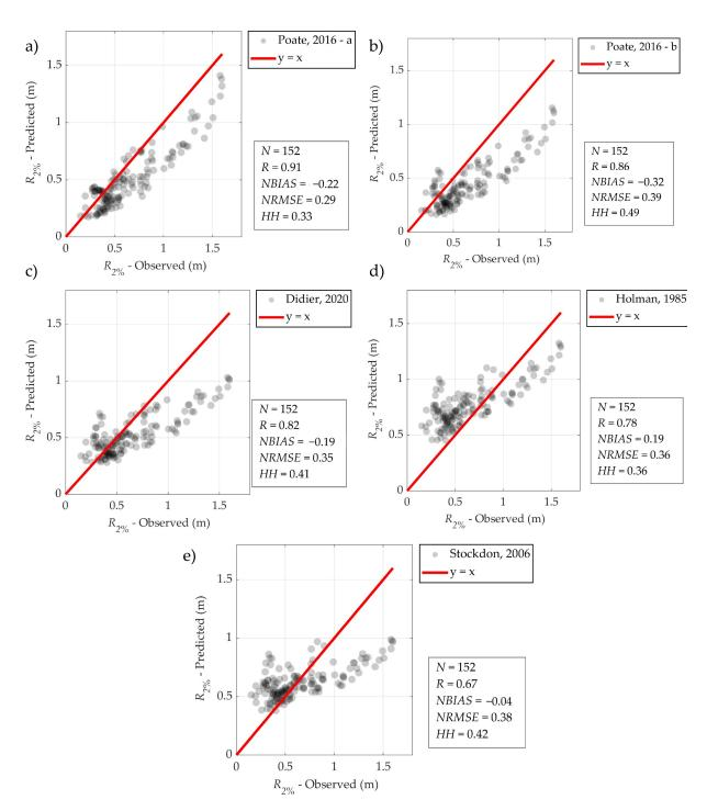
**Figure 7.** Comparison between observed runup values of fetch-limited pocket gravel beach Ploče and those predicted using the formulae outlined in Appendix B: (a) P16a, (b) P16b, (c) D20, (d) H85, (e) S06.
