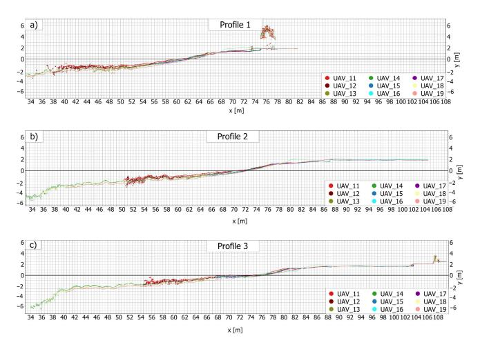
**Figure 2.** Cross shore profiles selected for the runup analysis; (a) the western profile position, which is shown on Figure 1d as profile 1; (b) the centerline profile position, which is shown on Figure 1d as profile 2; (c) the eastern profile position, which is shown on Figure 1d as profile 3; table showing the nine associated UAV surveys between 1 October 2020 and 26 February 2021 is in Appendix A.
