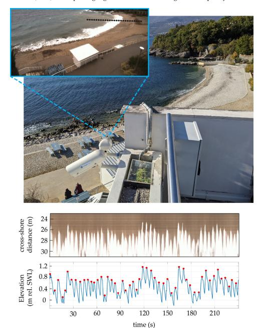
**Figure 3.** Position of the video monitoring system at the edge of the swimming pool complex at the beach site, one camera per beach cell; observed pixel cross-section of the acquired video gives the cross-shore distance time series of wave uprush, which ultimately results in the water elevation time series on the shoreline.
