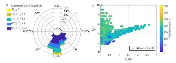
**Figure 5.** (a) The wave rose for the wave buoy during the measuring period (December 2019 to April 2021) in front of the Ploče beach; (b) scatter plot of significant wave heights against peak wave periods during the measuring period with wave direction as coloring.
