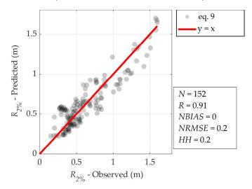
**Figure 10.** Comparison between the observed runup values on fetch-limited pocket beach Ploče and those predicted using the modified P16a equation by including the Goda peakedness parameter, *Qp* (Equation (9)).
