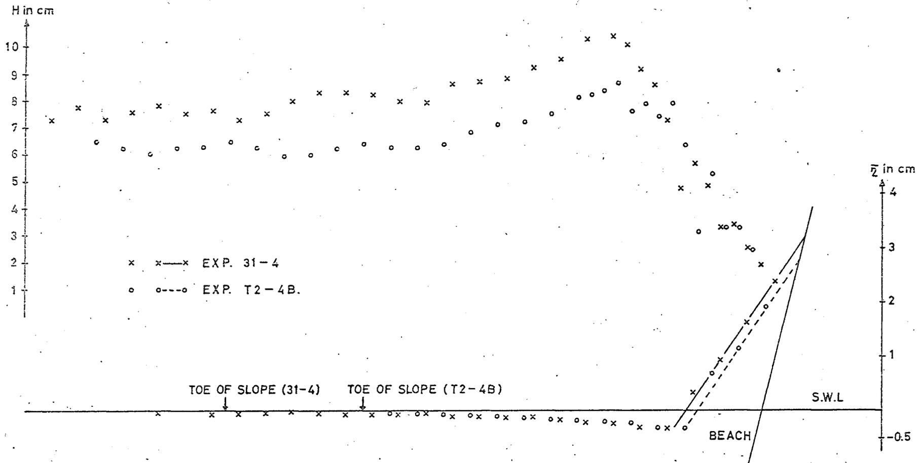
EXP. 31-4 :  $T=1.30$  sec ,  $h_1=40.1$  cm ,  $H_1=7.70$  cm ,  $TG \alpha = 0.10$  , WAVE TANK.
