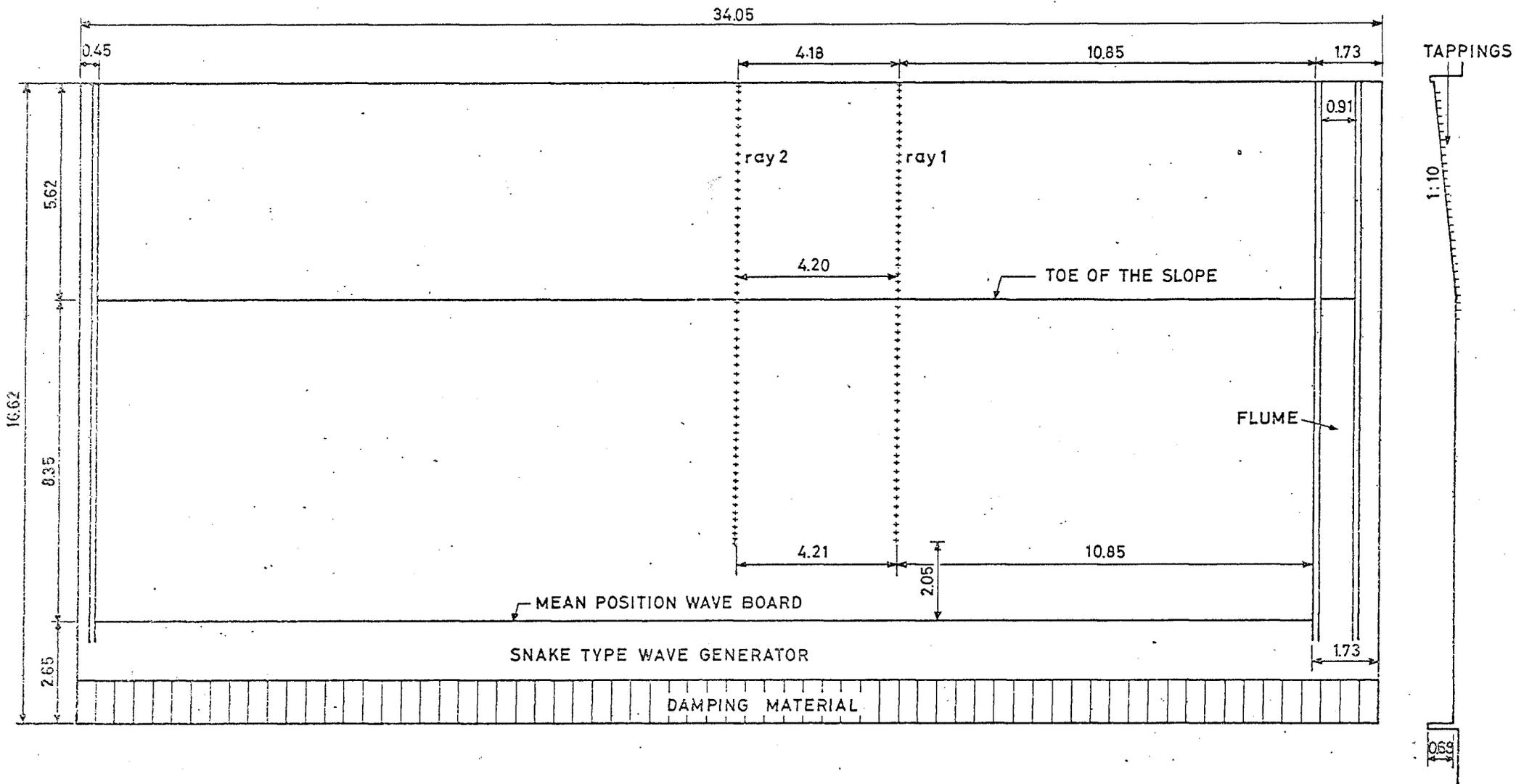
FIG.1 SCHEMATIC PLAN WAVE BASIN (MEASURES IN METERS)
