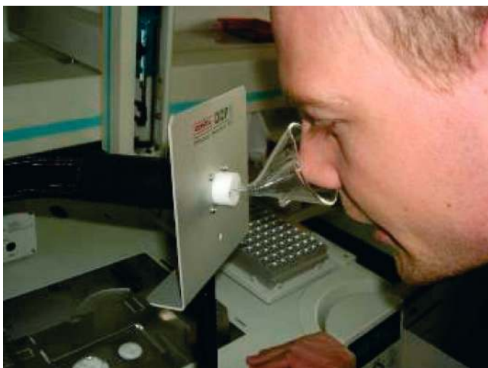
Fig. 19. Sensory detection of T&O compounds at the Sniff-Port; organoleptic detection port (ODP)
