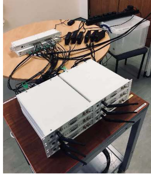
Fig. 5. Base station (USRP array).
