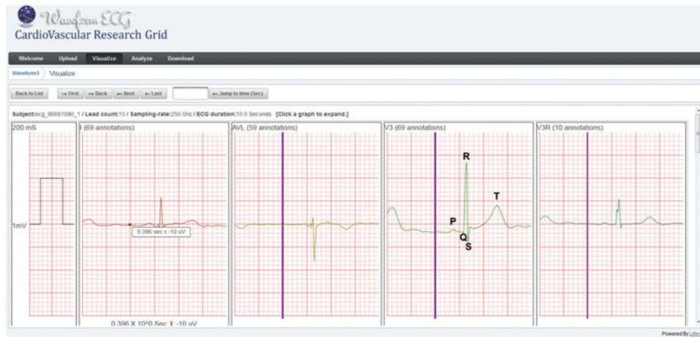
Figure 4. Multilead visualization interface. In the multilead display for 4 of the 15 leads from a GE Marquette Universal System for Electrocardiography (MUSE) XML upload, the vertical bar in 3 of the graphs represents the cursor location in the first graph. The bars move with the cursor and change focus as the cursor changes graphs.
