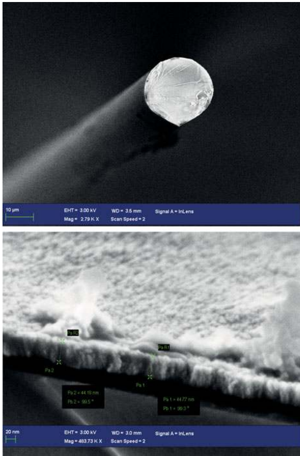
Fig. 10. SEM images of Sensor 2: Diameter 25 \mu\text{m} and ITO thin film 44 nm.
