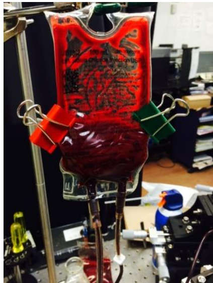
Figure 6.1 Prepared blood bag (blood source) containing the sheep blood. Air was completely removed to prevent any coagulation during the experiment. Generic paper clamps were also placed as shown as an extra safeguard to ensure no contact between blood and air.
