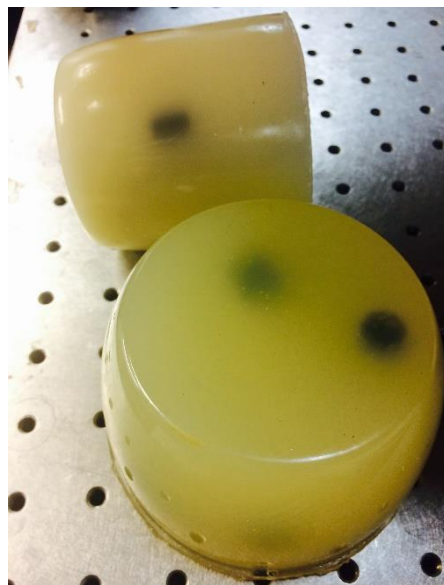
Figure 2.2 Human-breast-simulating PVCP plastisol samples with a few inclusions of higher absorption coefficient. Breast-tumor-simulating inclusion can be made of any kind of material as long as it has higher absorption than the background.
