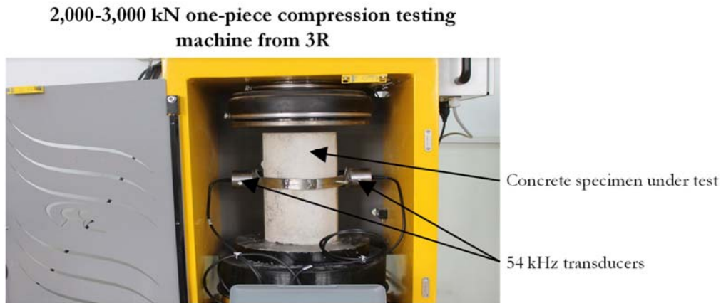
Figure 5: Experimental procedure for compressive tests.
