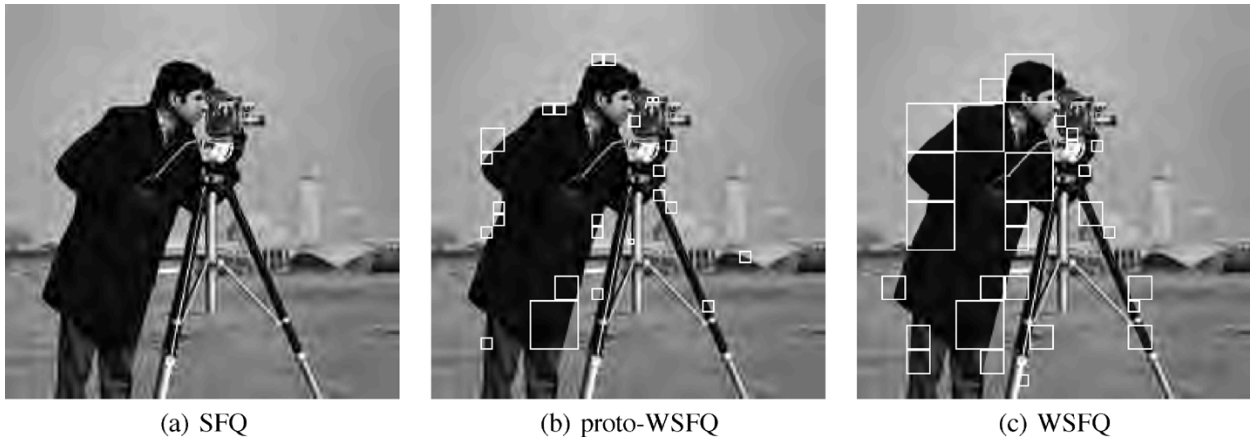
Fig. 6. Cameraman test image coded at 0.169 bpp. (a) SFQ results, PSNR 26.37 dB. (b) Proto-WSFQ results, PSNR 26.45 dB. (c) WSFQ results using enhanced wedgeprints, PSNR 26.73 dB. White boxes indicate the idealized support of each wedgeprint used in coding.
