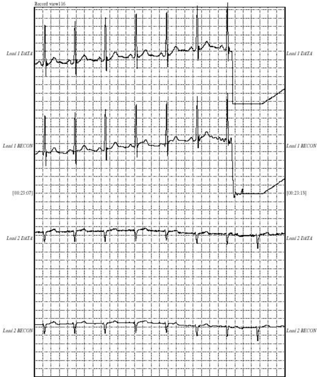
Figure 4: Original and reconstructed data from MIT-BIH Arrhythmia Database Record 116. Both leads from the database are shown, with original data traces above the corresponding reconstructed traces from data compressed by the Associated-Hermite algorithm. Performance of the algorithm over normal sinus data is seen to be excellent. At the end of a plot, lead 1 shows an artifact which is also captured in the reconstruction.
