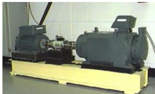
Figure 8. Test rig used in Case Western Reserve University Lab [41].
