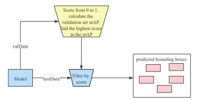
Figure 8. The flow chart of the OoF method.
