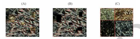
**Figure 3.** Illustrations of three data enhancement methods. (**A**) Cutout method; (**B**) cutmix method; (**C**) mosaic method.
