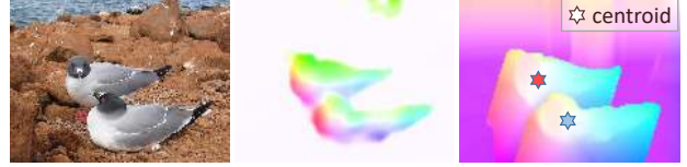
Figure 5. Detecting instance centroids. (left) Input image. (center) An initial displacement field. (right) A refined displacement field and detected centroids.
