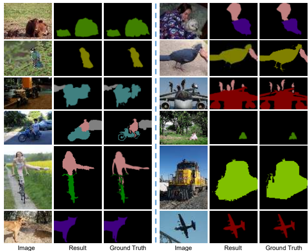
Figure 7. Qualitative segmentation results of the proposed framework on PASCAL VOC 2012 val set.
