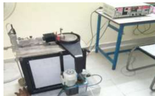
Fig. 3: Wear testing setup
