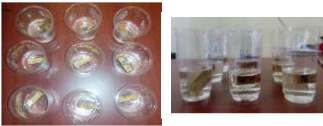
Fig. 4: Water absorption testing
