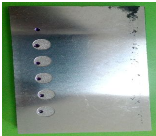
Fig 5. Brinell Hardness Test on OHNS machining surface
