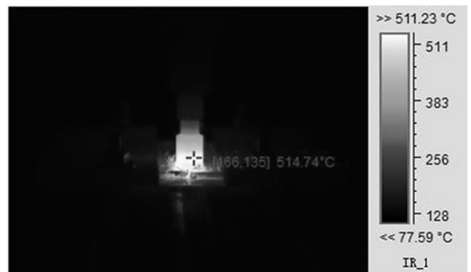
Fig. 3. Infrared image of FSW
