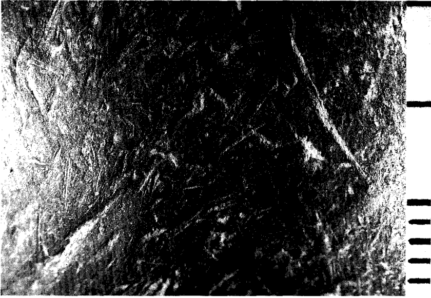
Figure 95 Part of a bit. Irregularly divided grooves in the steel, partly infilled, may point out a three-body wear process. Top of the bit at the left side of the photograph; a (small) scale-unit equals 1 mm
